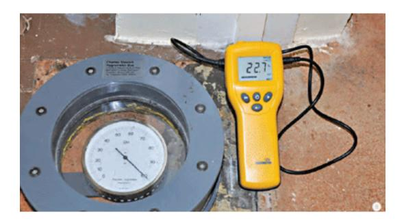
A mechanical hair hygrometer sealed to a solid ground supported solid floor after removing a single thermoplastic floor tile. The hygrometer rapidly recorded 100% relative humidity indicating that the solid floor was damp. This explained the timber damp reading of 22.7% to the bottom of the door lining (above the level at which timber will decay)
