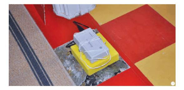
Purpose-made humidity box, sealed to the solid ground supported floor with hygrometer and temperature probe connected to a data capture device to measure the moisture profile of the solid floor (independent of the atmospheric conditions of the habitable rooms)
