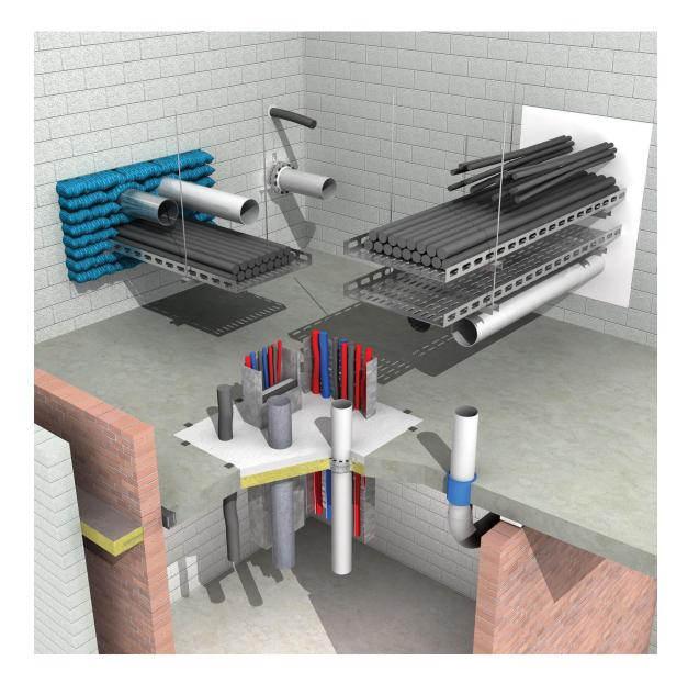
Figure 1. An overview of a fire-stopping application
